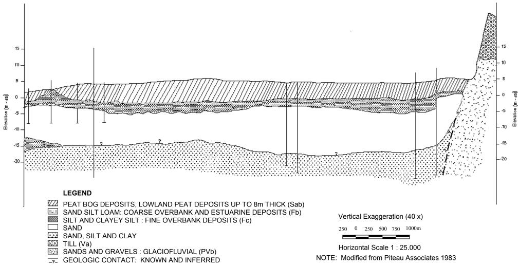
Figure 4.2 Surficial geology of the Burns Bog area, with the location of geologic section (A-A') as shown in Figure 4.1.
