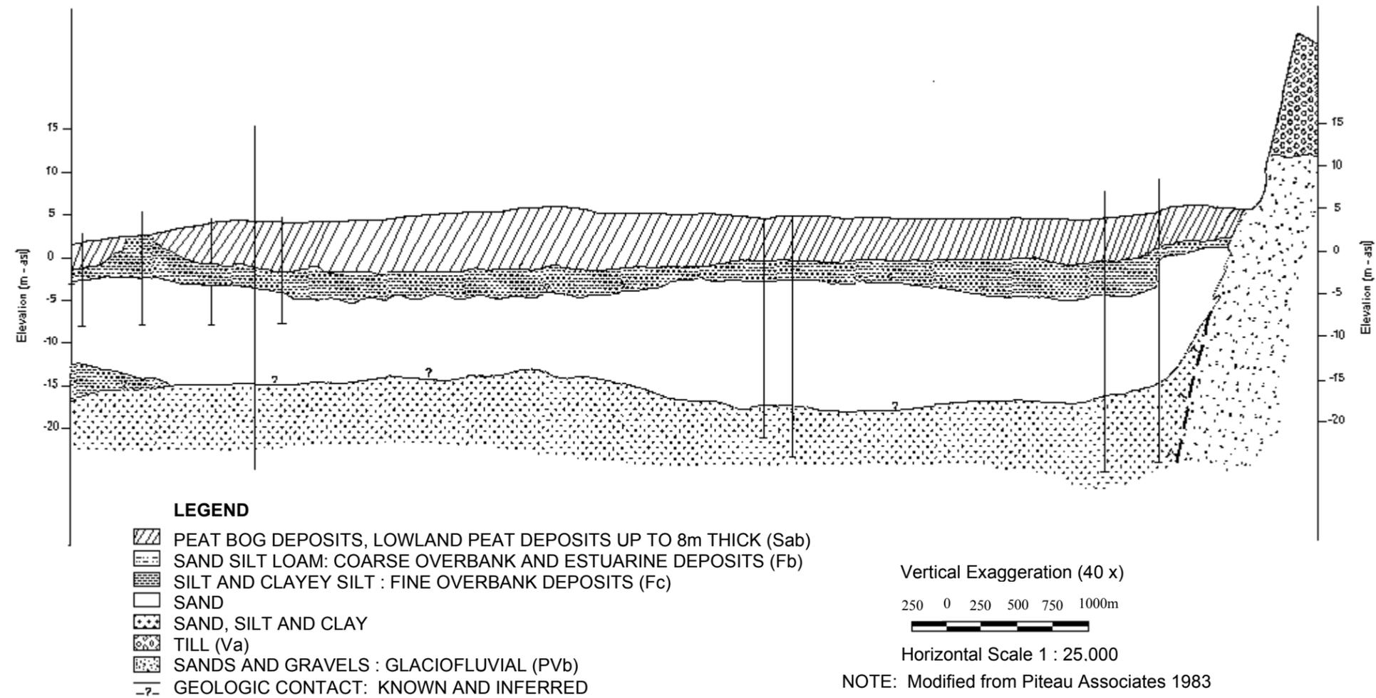
**Figure 4.2 Surficial geology of the Burns Bog area, with the location of geologic section (A-A') as shown in Figure 4.1.**
